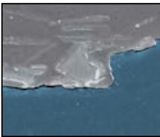
Paint simply lies on top of the substrate and may even bridge across pores in the metal. Since paint does not form a permanent bond to the substrate, it can easily release at very low stress levels.
