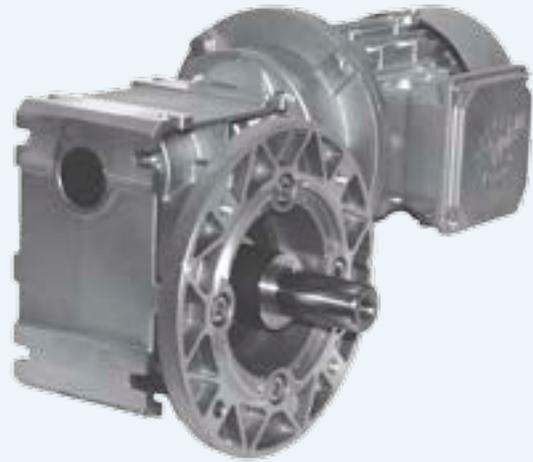
**Example:** Single reduction worm module SK 1SI50 with 50:1 ratio, 1 hp motor 230/460V with terminal box position 1, and conduit entry location I, plug-in solid shaft side A, B5 flange side A.
