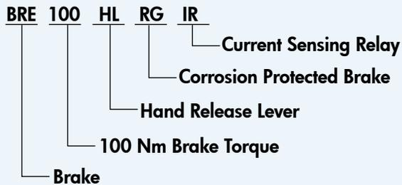
Brake, 100 Nm with a hand release lever, corrosion protected brake, and a current sensing relay.
