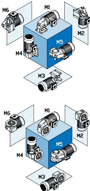
The gearbox mounting position is an important and often overlooked specification. The mounting position determines how much oil the gear reducer requires, in addition to determining the position of the oil drain, oil fill and vent on the gear drive. NORD offers six basic mounting positions. If your application requires a variation from the six basic mounting positions, please contact NORD.
