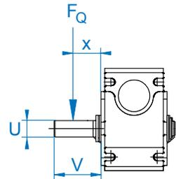
Overhung load [ $F_Q$ ] can be found in the gearmotor rating tables. Overhung load capacities should not exceed the values in the table to ensure long bearing life.
