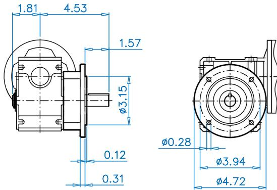
**SK 1SI40 VF (Plug-In Shaft, II Flange)**
