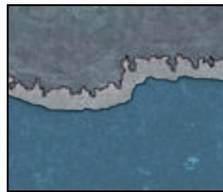
The NSD<sup>tupH</sup> process includes a base layer that is permanently bonded to the substrate and provides a powerful foundation for adhesion of the surface sealant. This foundation provides excellent roughness, is 6-7x harder than the aluminum substrate and up to 1000x harder than paint.
