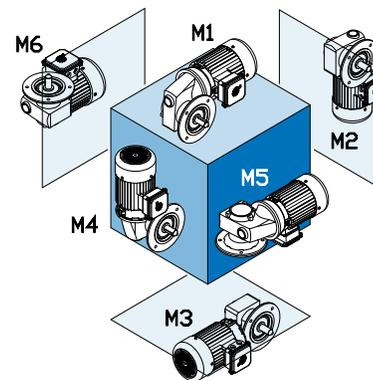
The gearbox mounting position is an important and often overlooked specification. The mounting position determines how much oil the gear reducer requires, in addition to determining the position of the oil drain, oil fill and vent on the gear drive. NORD offers six basic mounting positions. If your application requires a variation from the six basic mounting positions, please contact NORD.
