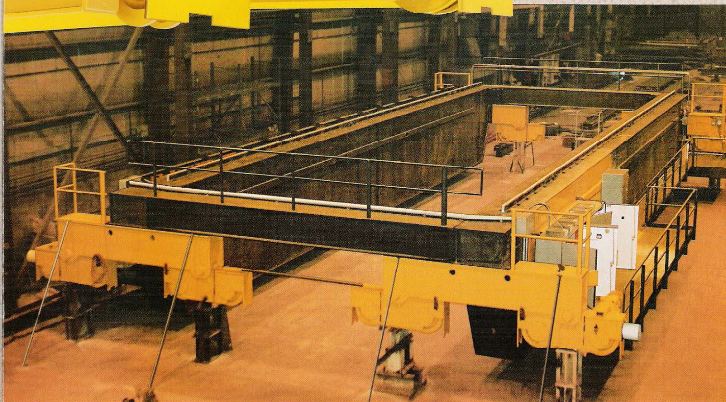
This 300/165 ton crane is being built by an ACE customer. ACE World Companies provided the trolley-hoist, end trucks, controls and designed the girders as well as the overall crane design.
