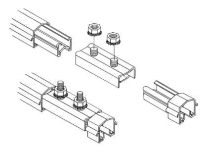
NOTE: A liberal coating of joint compound FS-JNJC is recommended on all mating faces that conduct current.
