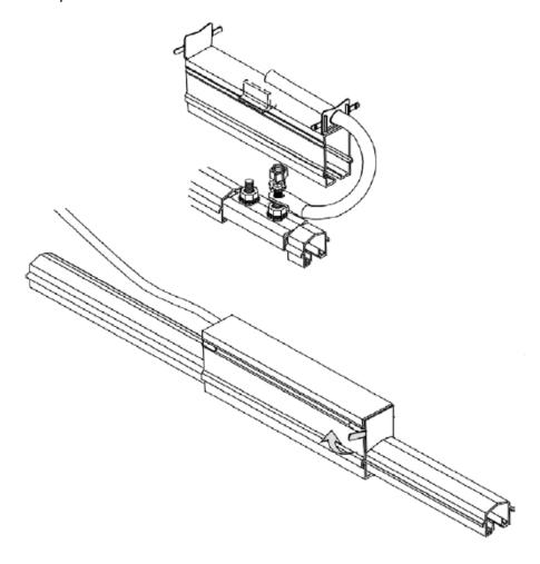
NOTE: A liberal coating of joint compound, FS-JNJC, is recommended on all mating faces that conduct current.
