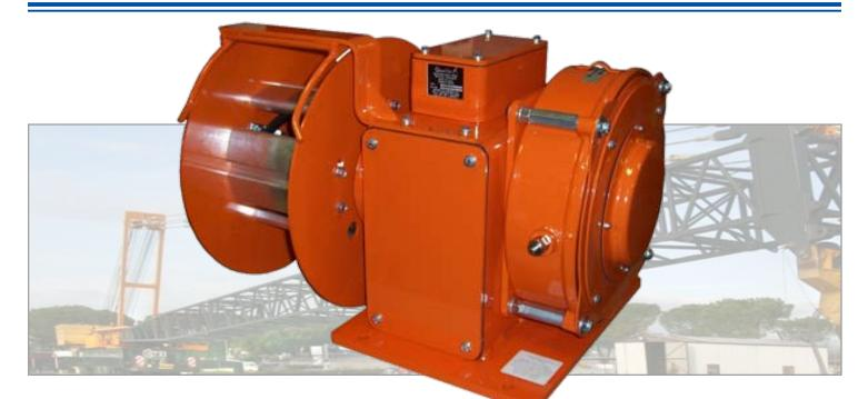
These compact, rugged **GLEASON SHO-101A REELS** have gained much favor with the scrap handling industry and manufacturers of magnet handling cranes. Designed to fit within the crane boom, it is the answer to magnet cable handling problems. Constructed entirely of steel with a powerful long-life main spring. Precision ball bearings are used throughout. Heavy cross section slip rings and copper-graphite brushes ensure electrical contact. Collector assembly rating - 2 pole, 75 amp, 600 volts.
