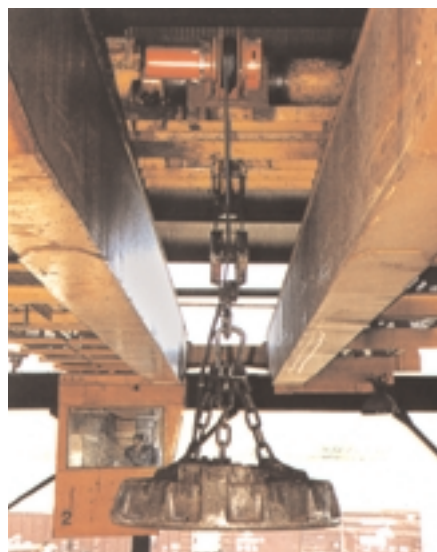
ON THE COVER: Typical Gleason Series "S" reel mounted on an overhead crane for heavy duty, high cycle, vertical lift service.
