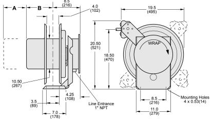
\* Wire size code is located in model number. Example: C16 - **A** 03 - F1105 (A - F possible)
