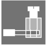
M12 plug-in connector in IP 67 available with crew or tension clamp connection
